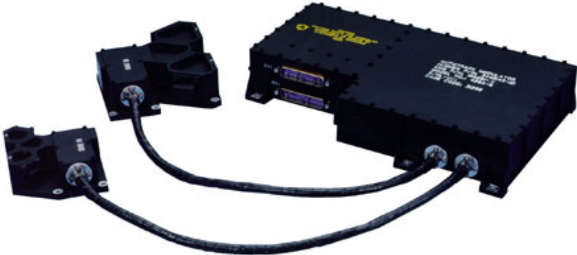
Figure 10. This phase shifter based autotrack modulator is currently flying on NASA's TDRS H, I, and J spacecraft. It consists of a single driver and control electronics box with two RF heads, one in K_u band and one in K_a band.
